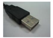
Figure 3: Type A USB connector.
